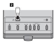
■ Press the USB source button to switch the audio source to USB.
